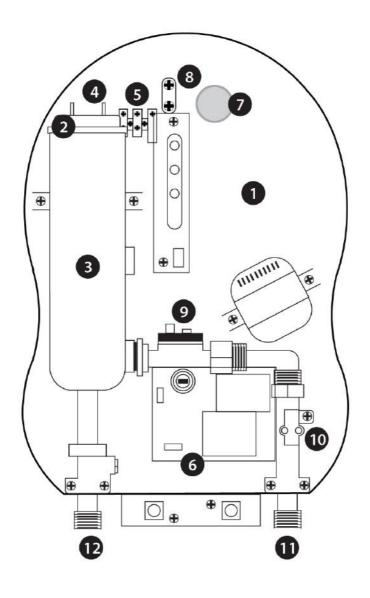
**Heater Base** 1 **Heating Element Heating Tank Thermal Cut-out Terminal Block Electronic Control Board**
